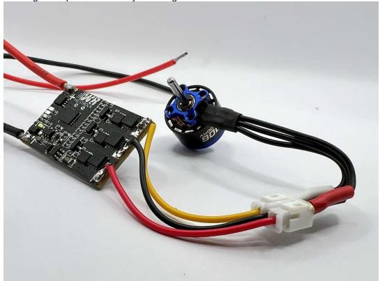
If your motor rotates backwards switch the connections you made of the outer wires. If you carefully follow the wiring in the photo you will have the correct rotation.
